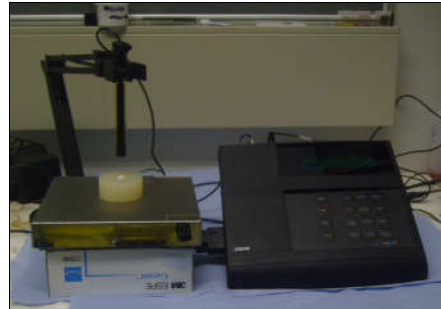
Figure-2: Fluoride release measured by Ion Electrode
